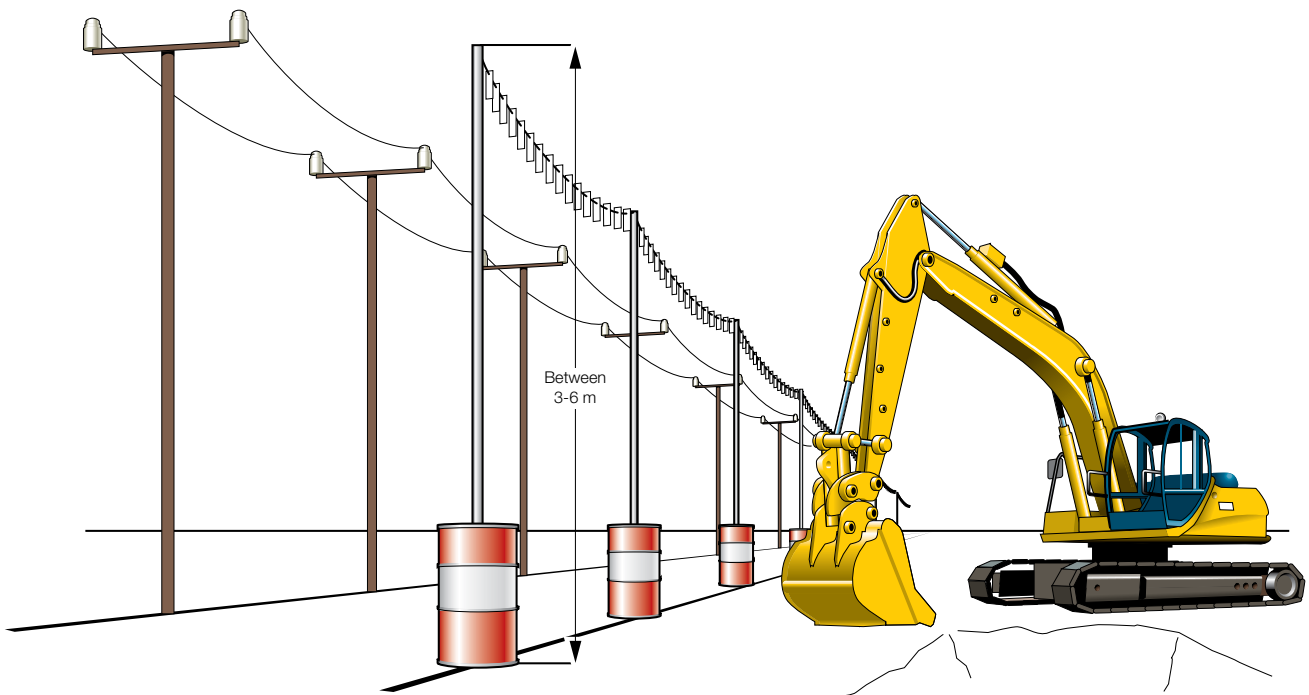
Figure 49 Ground-level barrier for plant working near an overhead power line
