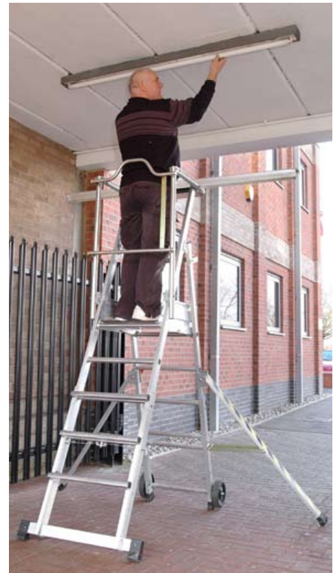
Figure 22 Working platform stepladder
